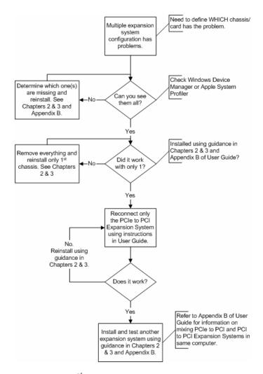
Problems with 3<sup>rd</sup> Party cards might only be trackable once you have identified the expansion system containing the problem card. Remember, it may be necessary to identify the PCIe/PCI Slot that the Host Interface Card is in before you can properly identify the correct expansion chassis and ultimately the card. Obviously, this is only an issue if you have multiples of the same type of card installed.
